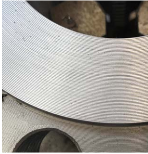
Single line gramophone groove (50 grooves per 1 inch)
