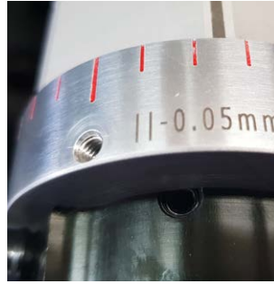
Graduation of the tool setting to the desired depth of cut.
